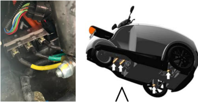
Water get inside after cutting phase wire shield
